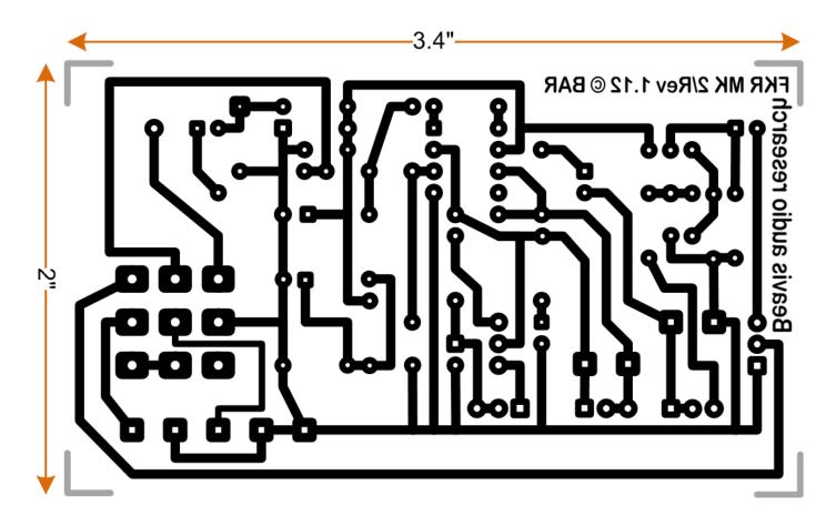
To get the size right, print the PCB out on paper first. Take a 8-pin DIP chip and line it up with the holes for U1 as shown in the parts layout below. Resize the image and reprint until you get the IC pins to line up exactly. Use the 3PDT switch as another reference point. Once everything lines up \*exactly\* you should have the right size.
